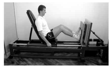
A foot-platform fixed to the frame by strain-gauge transducers and data was collected at 2000 Hz using interface box with an analog to digital card (National Instruments, Austin, TX, USA). During later off-line analysis the trials were selected and the force signal was filtered by a digital fourth order recursive low-pass filter, using a cutoff frequency of 50 Hz. Thereafter, data was processed using a PC.
